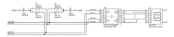
Figure 1: LAN Interface for DNP/5280 Rev. 1.1
