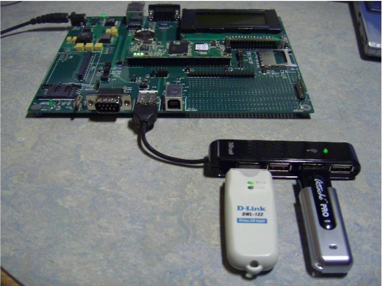
Picture 1: DNP9200 + eval board SK23, external mini USB2.0 Hub with a 11Mbps WLAN USB Adapter and 1GB high speed(192x) USB SWAP device.
