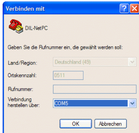
Figure 6: Direct connection setup with HyperTerminal
