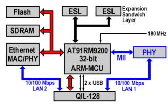
Block diagram ADNP/9200: The DIL/NetPC ADNP/9200 comes with two 10/100 Ethernet LAN interface, 20-bit GPIO, 1 x SPI, 3 x UARTs, 2 x USB Host port, 1 x USB Device port and Expansion Sandwich Layer (ELS) connector. The 16-bit bus interface (available over the QIL-128 connector) supports the connection to external chips and devices. The main application area of the ADNP/9200 is the new field of Ethernet-to-WSN (Wireless Sensor Network) gateways for industrial and laboratory environments.
